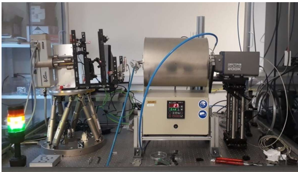
Figure 4.3 Photo of the in-situ GIWAXS measurement setup in the laboratory.
