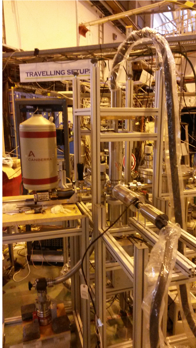
Figure 2: Photograph of TATRA spectrometer at ISOLDE LA1 beamline with all detectors mounted.
